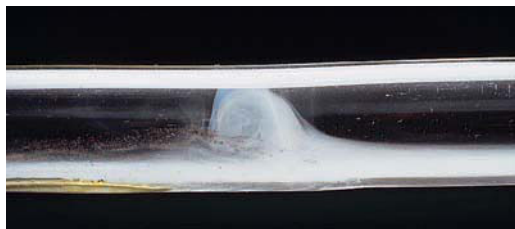
When \text{HCl}(g) and \text{NH}_3(g) meet in a tube, a white ring of \text{NH}_4\text{Cl}(s) forms.
