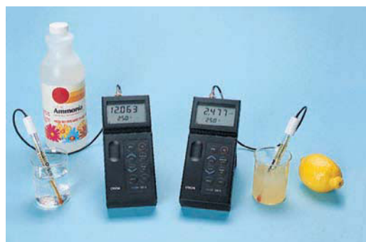
FIGURE 14.9 pH meters are used to measure acidity.
